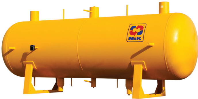
Ammonia liquid separators NLS Diameter range up to 2 m Length range up to 12 m Temperature range -50 to 50 °C Working pressure range up to 20 bar
