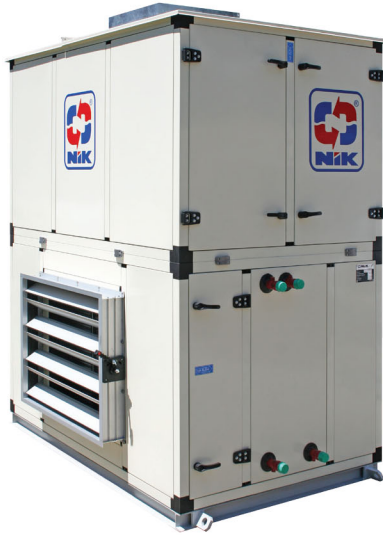
Standing air handling unit NAH-S Cooling capacity range 33 to 675 kW Heating capacity range 63 to 1310 kW Air flow range 3400 to 68000 m3/hr
