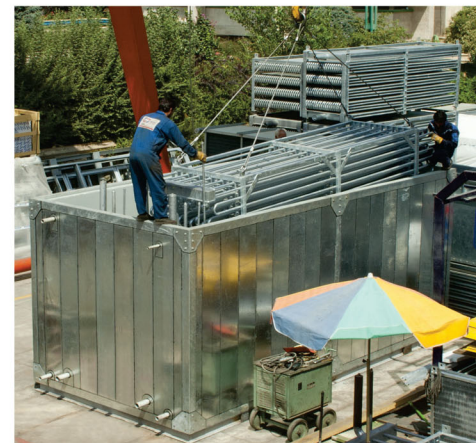
Plate freezers NPF Capacity range 600 to 2000 kg/run
