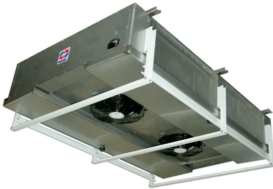
Dual discharge ammonia unit coolers AND-D Capacity range 3.5 to 65 kW Fan diameter 400,450,500, or 560 mm NO. of fans 1, 2 or 3 fans Fin spacing 6,8,10,12,15 or 12/15
