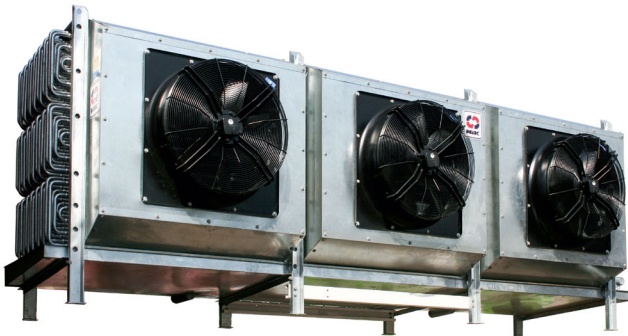
Industrial ammonia unit coolers AND-I Capacity range 48 to 203.3 kW Fan diameter 630 or 710 mm NO. of fans 2 to 5 fans Fin spacing 6,8,10,12,15 or 12/15
