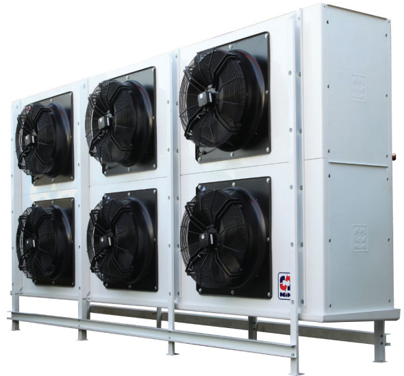
Matrix type tunnel freezer NBT-M Capacity Range 29 to 232 kW Fan diameter 630 or 710 mm NO. of fans 2, up to 8 fans Fin spacing 8 or 10 mm
