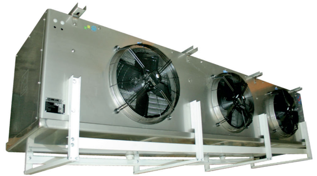
Commercial ammonia unit coolers AND-C Capacity range 4 to 100.9 kW Fan diameter 450,500 or 560 mm NO. of fans 2 to 5 fans Fin spacing 6,8,10,12,15 or 12/15
