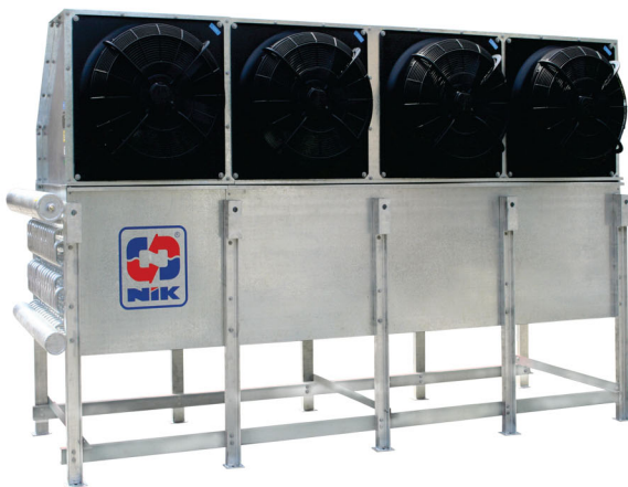
Tunnel freezer ammonia unit coolers AND-T Capacity range 48 to 295 kW Fan diameter 630 or 710 mm NO. of fans 2,3,4 or 5 fans Fin spacing 6,8,10,12,15 or 12/15
