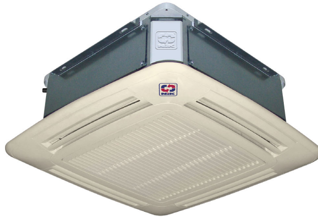
Four way cassette fan coil NFC-F Cooling capacity range 1.6 to 10.9 kW Heating capacity range 2.5 to 14.1 kW Air flow range 330 to 1750 m 3 /hr
